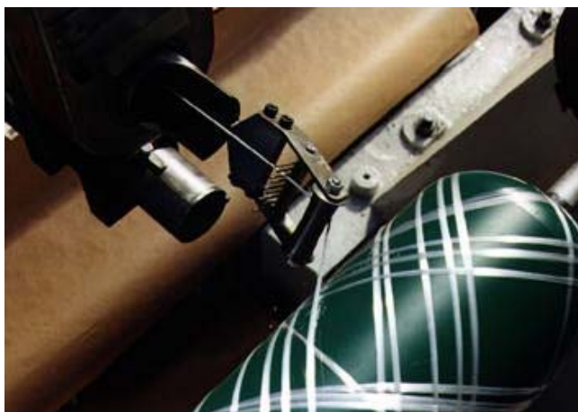
Figure 3: Close-up of a pay-out eye and mandrel
