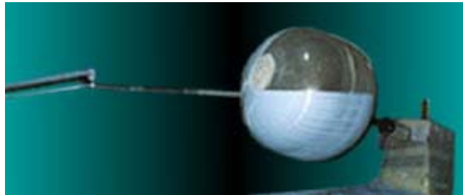
Figure 2: Winding a short pressure vessel
